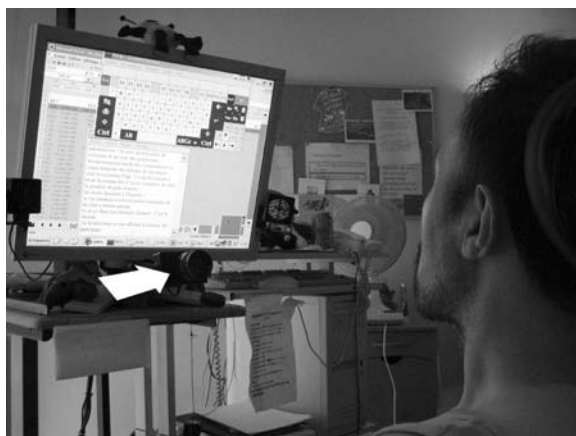
Fig. 4. A locked-in person updates the database of ALIS, moving the cursor on screen by eye movements. An infrared camera (white arrow) mounted below the monitor observes one of the user's eyes, an image processing software continually analyzes the video image of the eye and determines where the user is looking on the screen. The user looks at a virtual keyboard that is displayed on the monitor and uses his eye as a computer-mouse. To "click" he looks at the key for a specified period of time (typically a fraction of a second) or blinks. An array of menu keys allow the user to control his environment, use a speech synthesizer, browse the worldwide web or send electronic mail independently (picture used with kind permission from DT). With a similar device Philippe Vigand, locked-in since 1990, has written a testimony of his LIS experience in an astonishing book Putain de silence (1997) translated as Only the Eyes Say Yes (2000). Photograph by S. Laureys.
